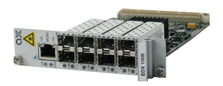
The EDX1006sync is designed as synchronous media converter and aggregation devices in provider's network and edge. A wide bunch of different optical interfaces are supported on LAN and WAN side of the unit. All types of SFPs are supported and so an universal synchronous converter/repeater for wavelength, fibre-mode, distance and speed can be setup. The clocking information provided on one WAN-link can be derived on the EDX1006sync and forwarded to all the other ports.
