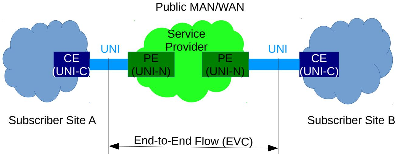
Figure 3: Architecture Reference Model, Subscriber View
