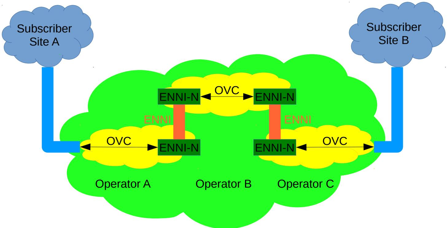
Figure 4: Architecture Reference Model: Service Provider View
