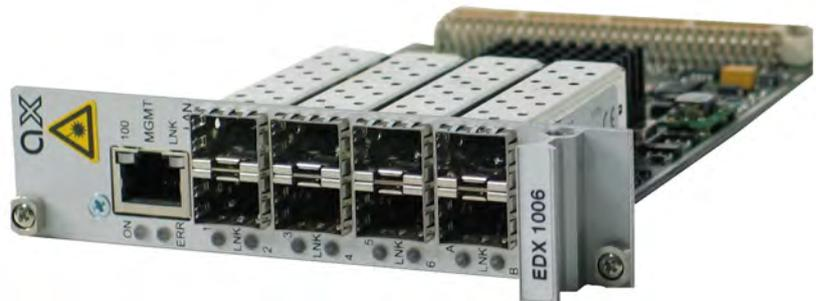
The EDX1006sync is designed as synchronous media converter and aggregation devices in provider's network and edge. A wide bunch of different optical interfaces are supported on LAN and WAN side of the unit. All types of SFPs are supported and so an universal synchronous converter/repeater for wavelength, fibre-mode, distance and speed can be setup. The clocking information provided on one WAN-link can be derived on the EDX1006sync and forwarded to all the other ports.
