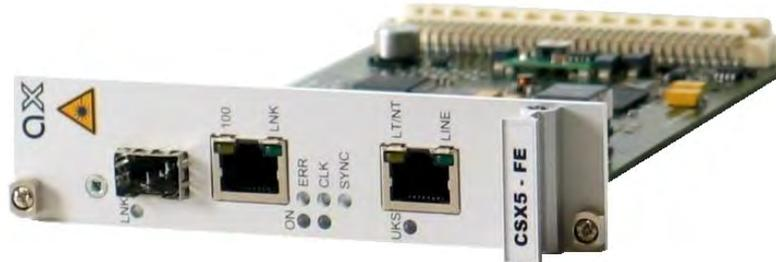
The CSX product family provides symmetrical high speed transmission on copper lines, based on G.SHDSL. It offers cost-efficient, flexible and reliable services for SME and SOHO customers as well as in campus applications. The CSX family is fully-managed and can be operated in a chassis as well as in a desktop housing. G.SHDSL is the best solution to quickly provide cost-effective, high-speed network service for users who need symmetrical connections.
